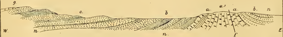
Sketch section from the Bil. scarp to the Gabbar plain g. Gaj. n. Nari beds. f. Fault.
